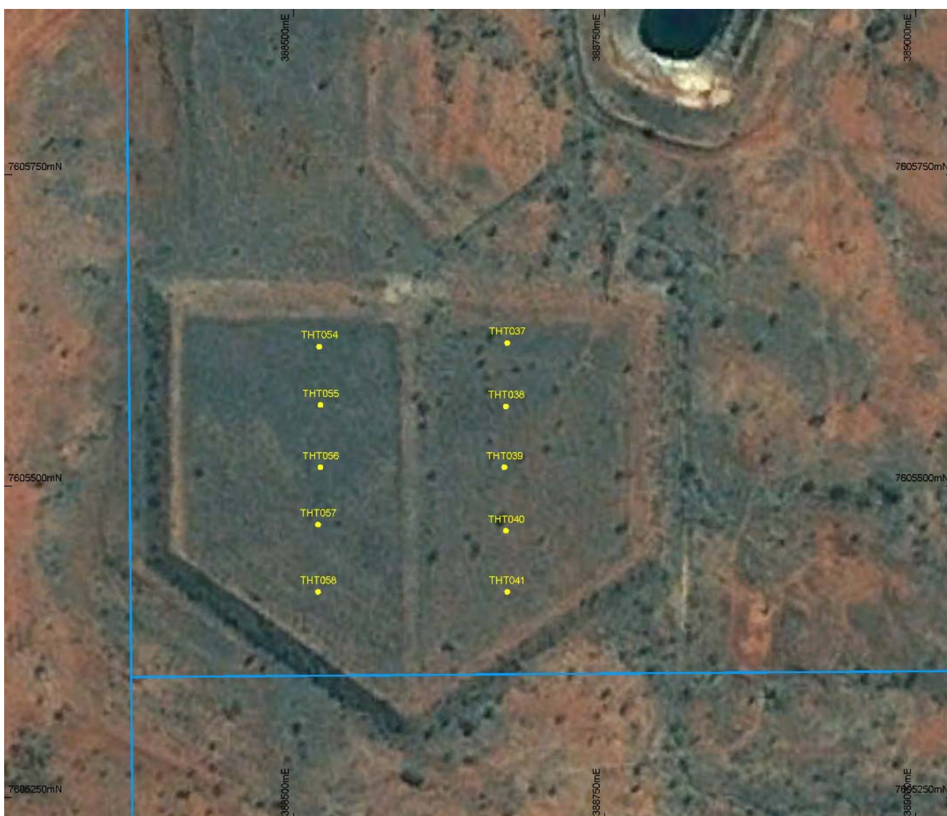
Figure 1: Location Map Tick Hill Gold Project – Tailings Dam bulk sample drill holes on Google Earth
